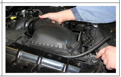
5.Remove the top bolt from the lower heat shield (10mm) then the other two (8mm) bolts to release the lower heat shield.
