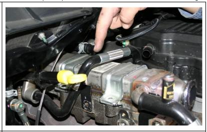
13.Remove the coolers two rear bolts that attach it to the exhaust system (15mm)
