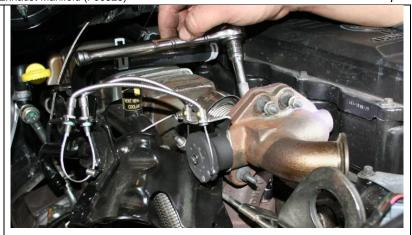
9.Remove the EGR flow direction valve from the vehicle.
