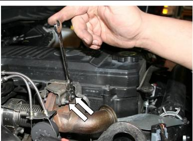
4.Remove the air box and intake hose. Remove the air filter inlet hose from the turbo inlet.
