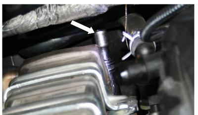
14. Prop the cooler above the studs and push towards the cab holding the other coolant hose to release the oring fitting to remove the cooler from the vehicle.
