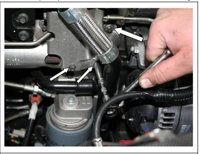
6.Remove the three bolts for the stepper motor bracket (10 mm) socket and prop the bracket on the cooler.
