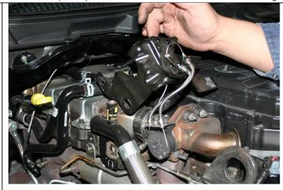
7.Loosen the clamp (11mm) that connects the EGR Flow Direction Valve to the cooler and slide the clamp towards the valve.
