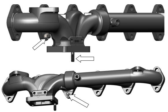
Arrow point to the locations of 30mm studs. All 25mm studs are installed in the EGR ports.
